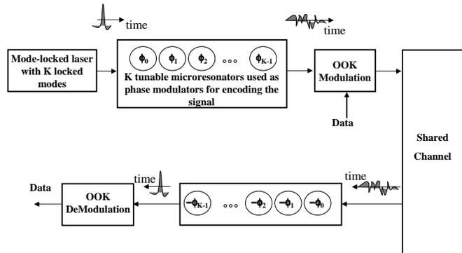
Fig. 4. Phase Encoding OCDMA system with Coherent Source.
