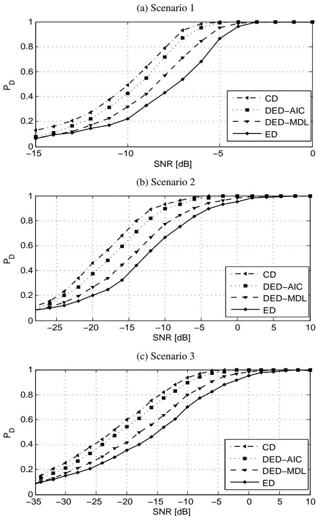
FIGURE 2. Performance evaluation of the DED detector in terms of PU signal detection using an DVB-T OFDM PU system: Probability of detection versus SNR curves with  $P_{FA} = 0.05$ , sensing time =  $1.12ms$  and  $p = 2048$ .
