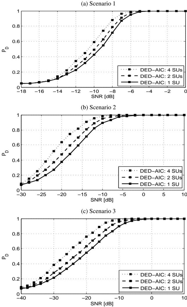
FIGURE 3. Performance evaluation of the DED detector in terms of PU signal detection in cooperative way using an DVB-T OFDM primary user system: Probability of detection versus SNR curves with  $P_{FA} = 0.05$ , sensing time =  $1.12ms$  and  $p = 2048$ .
