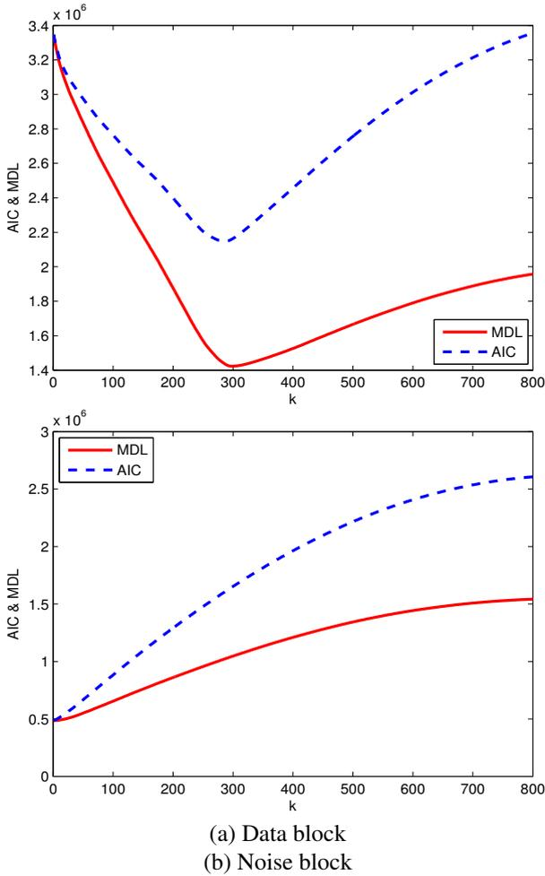
FIGURE 1. Akaike information criterion and minimum description length of captured noise block samples and data block samples using an UMTS signal.
