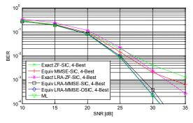
Figure 4- Uncoded BER,  $4 \times 4$  complex Rayleigh channel, 16-QAM modulation on each layer, K=4
