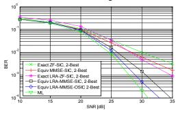
Figure 3- Uncoded BER,  $4 \times 4$  complex Rayleigh channel, 16-QAM modulation on each layer, K=2
