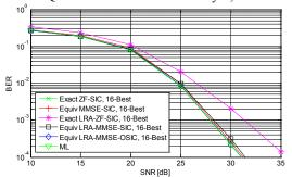
Figure 5- Uncoded BER,  $4 \times 4$  complex Rayleigh channel, 16-QAM modulation on each layer, K=16
