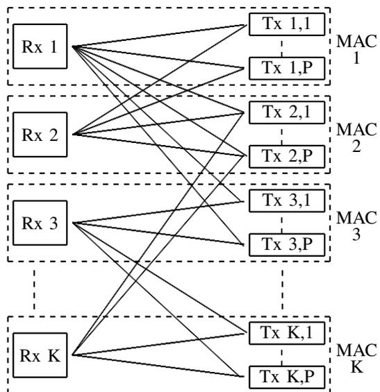
Fig. 1. Example connectivity graph in a partially connected interfering MACs model. Lines represent channels with non-zero coefficients.
