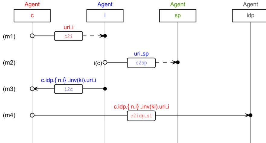
Figure 10: Attack on the SAML-based SSO for Google Apps despite signature on the authentication request
