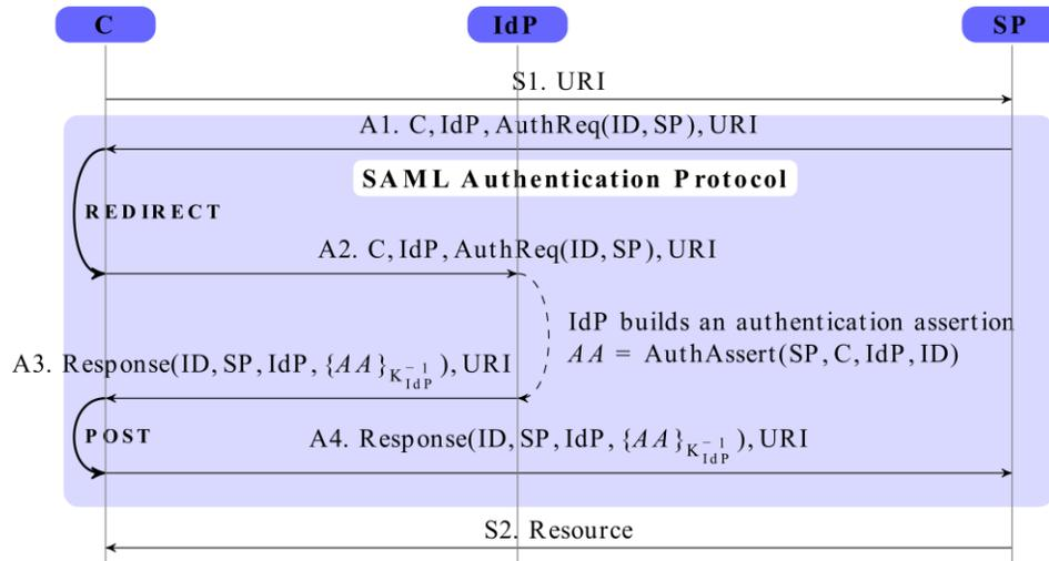
Figure 2. SP-initiated SSO with redirect/POST bindings
