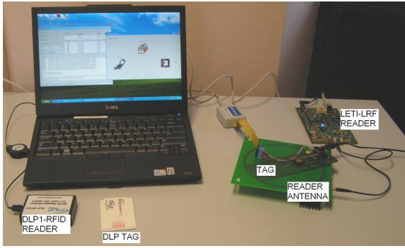
Figure 2: Hardware setup used for  $F_f$  integration
