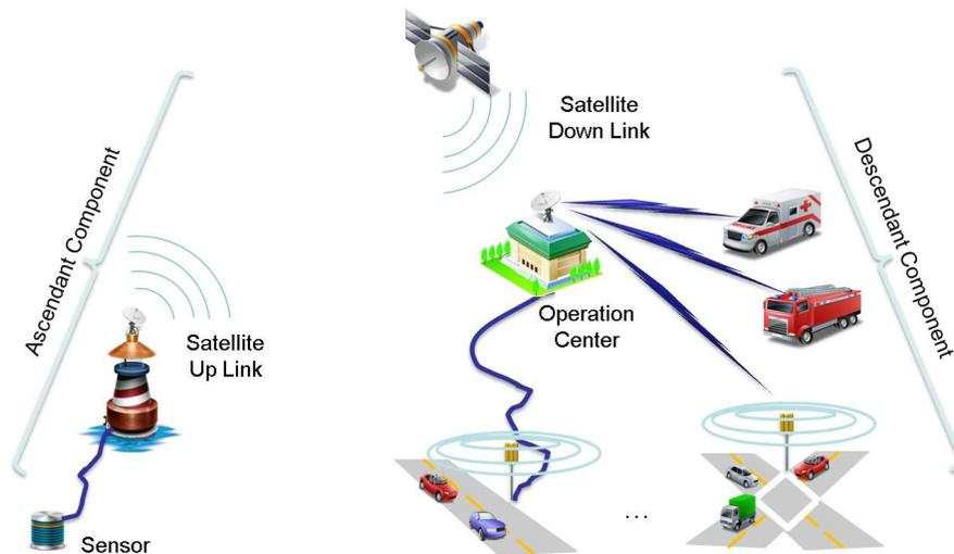
*Figure 4 - Ratcom project main architecture*
