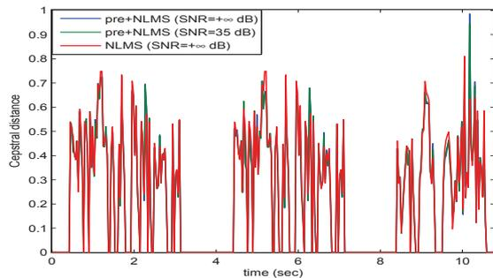
Figure 4: Cepstral distance between the far-end signal and the loudspeaker output.
