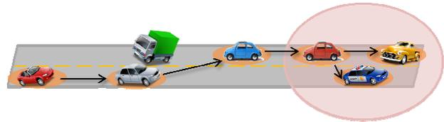
Figure 3. GeoBroadcast type of V2V communication
