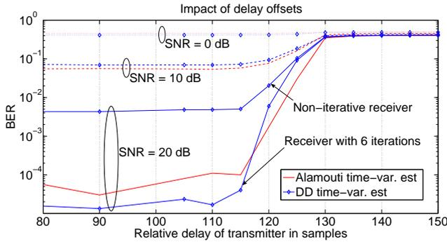
Fig. 6. BER performance of distributed Alamouti and delay diversity STC under different timing offsets of the nodes;  $f_{\text{off},1} = -250$  Hz,  $f_{\text{off},2} = 500$  Hz.
