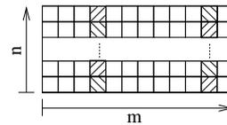
Fig. 4. Pilots are marked with diagonal lines. For the Alamouti scheme, orthogonal pilots are used (indicated by a different pattern), blank squares correspond to data subcarriers. The subcarriers with  $n \notin \{106, \dots, 405\}$  are used as guard band.
