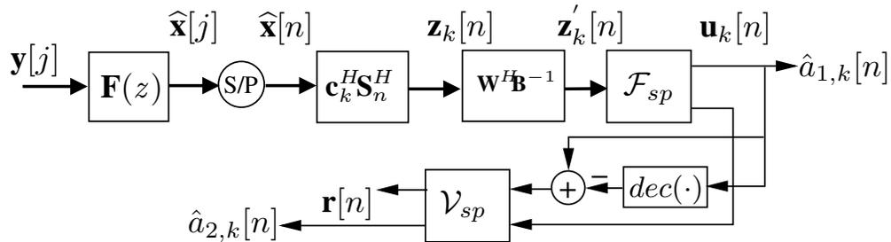
Figure 1.5: Chip LMMSE equalizer/correlator followed by spatial MMSE and symbol-level SIC for stream 2.
