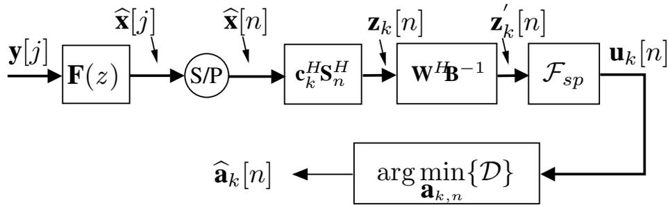
Figure 1.6: Chip LMMSE equalizer/correlator followed by spatial MMSE and joint detection.
