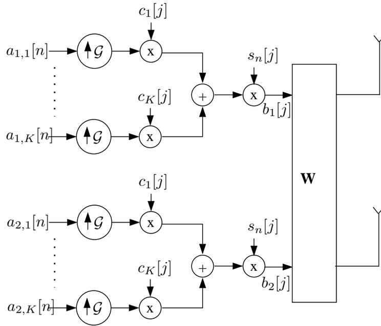
Figure 1.11: Multiuser D-TxAA transmit signal model.
