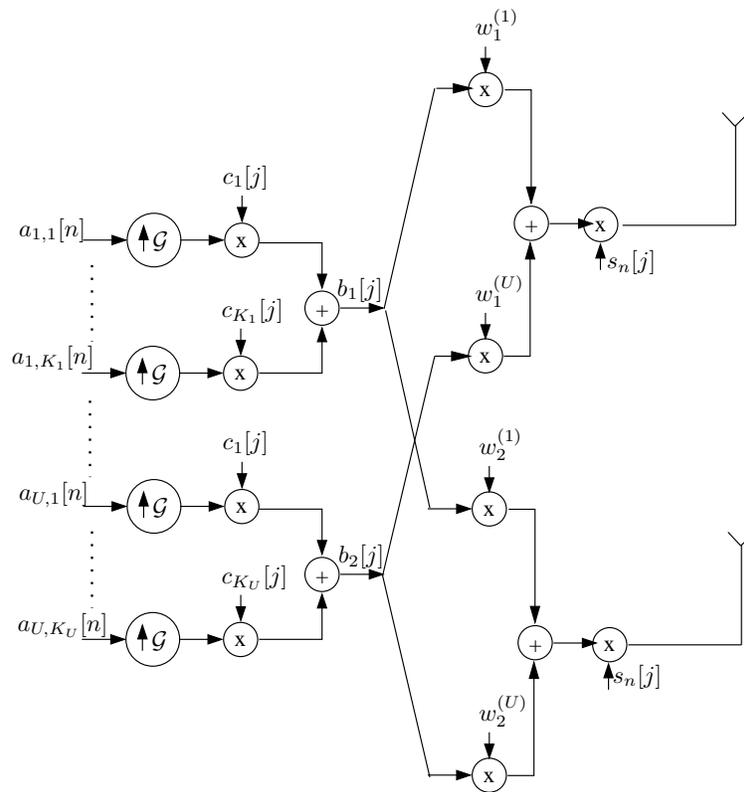
Figure 1.10: Multiuser TxAA transmit signal model.
