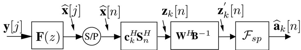
Figure 1.4: Chip LMMSE equalizer and correlator followed by symbol-level (spatial) MMSE.
