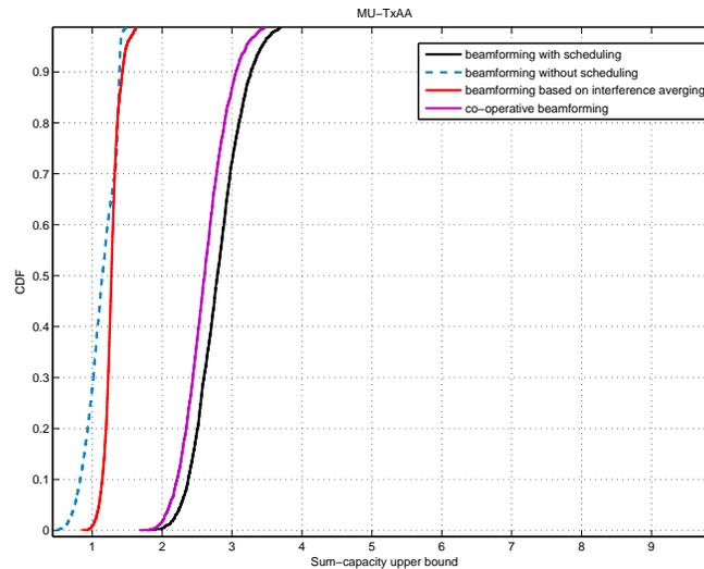
Figure 1.12: Performance of different beamforming schemes for MU-TxAA.
