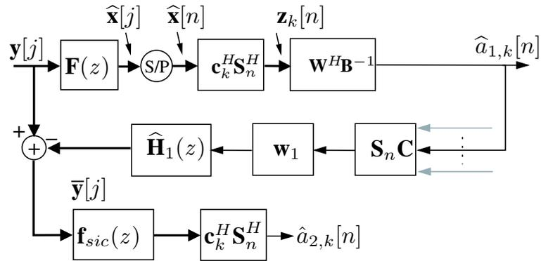
Figure 1.3: Chip LMMSE equalizer/correlator and chip-level SIC for stream 2.
