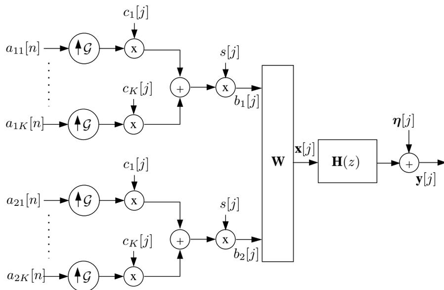
Figure 1.1: MIMO signal model with precoding.
