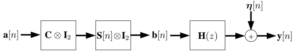
Figure 1.8: MIMO TX signal model.
