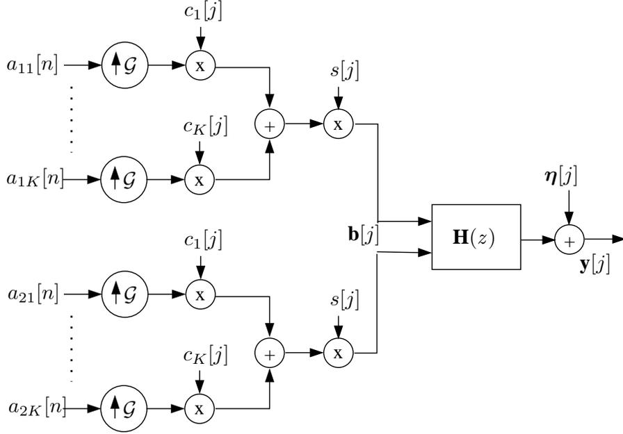
Figure 1.7: MIMO signal model without precoding.
