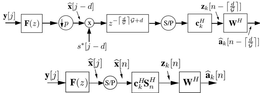
Figure 1.2: LMMSE equalizer and correlator. The second figure is a simplified representation used as chip-equalizer /correlator front-end stage for other receiver structures.
