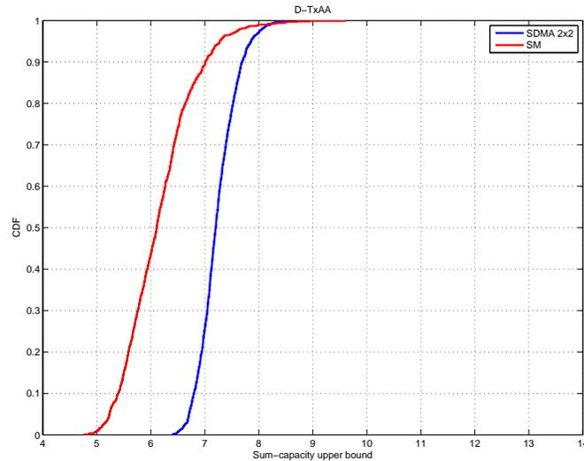
Figure 1.13: DL sum-capacity for MU-D-TxAA.
