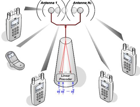
Fig. 1. MU-MIMO system model.
