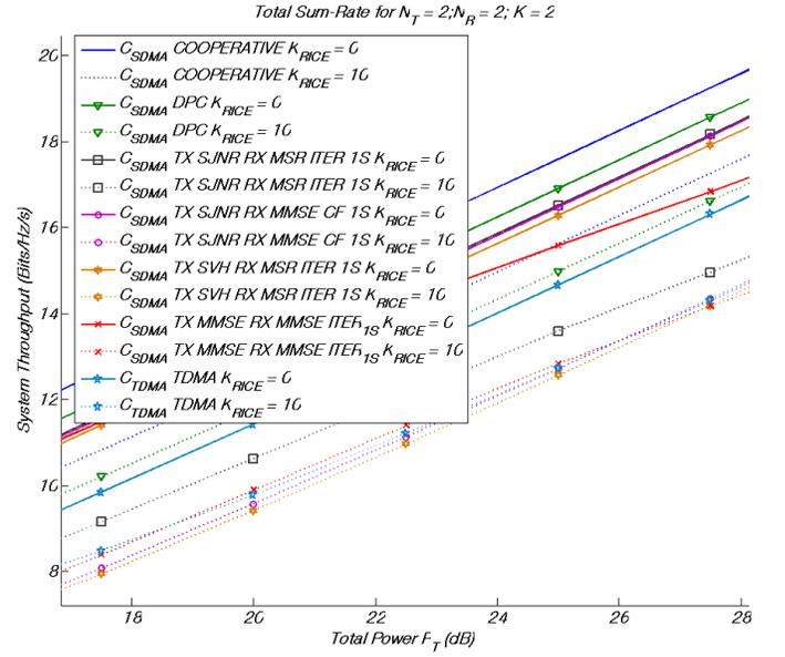
Fig. 4. Throughput as a function of total transmit power  $P_T$  for  $N_T = 2$ ,  $N_R = 2$  and  $K = 2$ .
