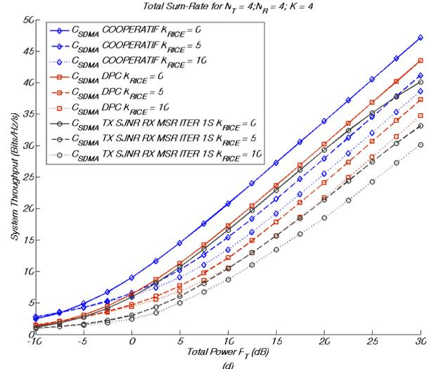
Fig. 2. Throughput as a function of total transmit power  $P_T$  for  $N_T = 4, N_R = 4$  and  $K = 4$ .
