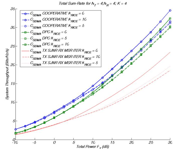
Fig. 5. Throughput as a function of total transmit power  $P_T$  for  $N_T = 4$ ,  $N_R = 4$  and  $K = 4$  with  $\theta$  channel.
