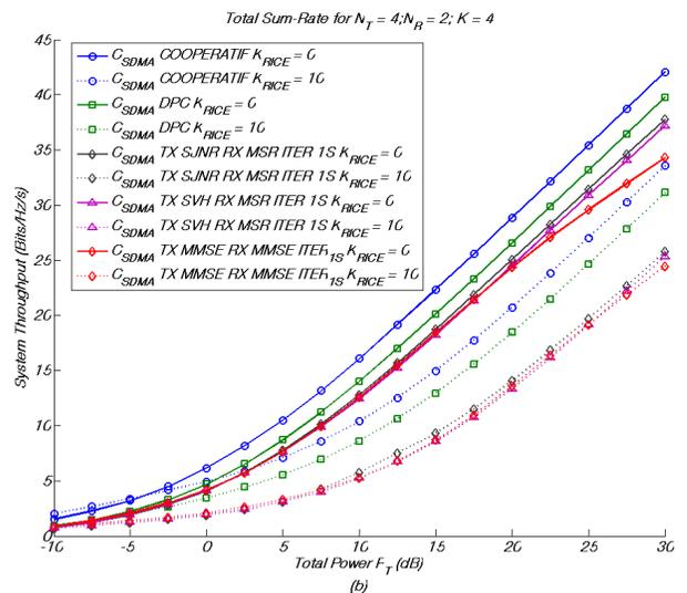
Fig. 3. Throughput as a function of total transmit power  $P_T$  for  $N_T = 4, N_R = 2$  and  $K = 4$ .
