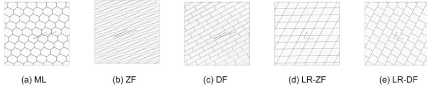
Figure 3.16: Undisturbed received signals and decision regions of: (a) Maximum-Likelihood, (b) Linear ZF, (c) Decision-Feedback, (d) Lattice-Reduction aided ZF and (e) Lattice-Reduction aided Decision-Feedback detection.
