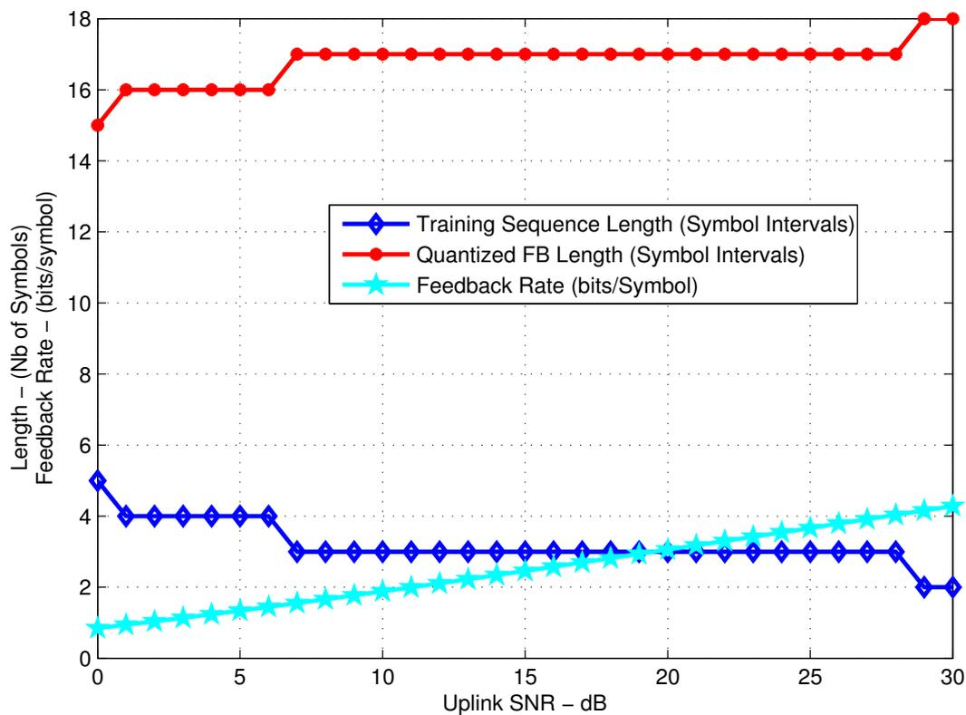
Fig. 4. Optimal Lengths and Outage Rate:  $T_{fb} = 20$  and  $M = 4$ . With increase in SNR, both the length of the quantized feedback interval  $T_q$  and the outage rate  $b$  increase gradually.
