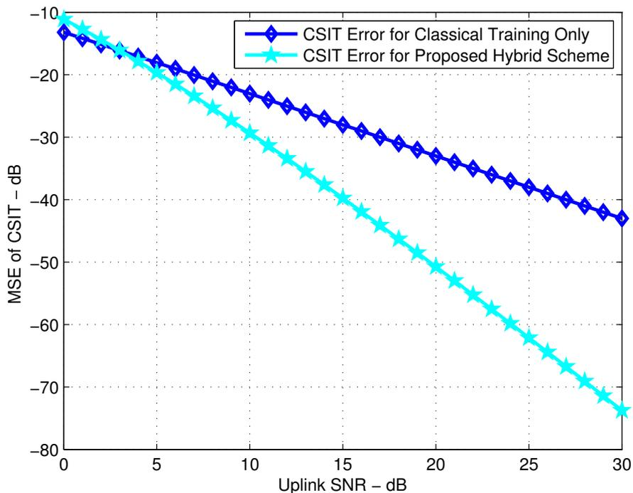
Fig. 3. Mean-Square CSIT Errors with perfect CSIR:  $T_{fb} = 20$  and  $M = 4$ . The novel hybrid scheme performs much better than the classical training based CSIT acquisition. Gains are significant even with naive use of practical constellations without any coding.
