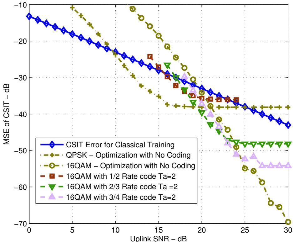
Fig. 8. Mean-Square CSIT Errors with Convolutional Coding:  $T_{fb} = 20$  and  $M = 4$ . At certain SNR intervals, coding strategy performs better than no coding optimal resource split outcome.
