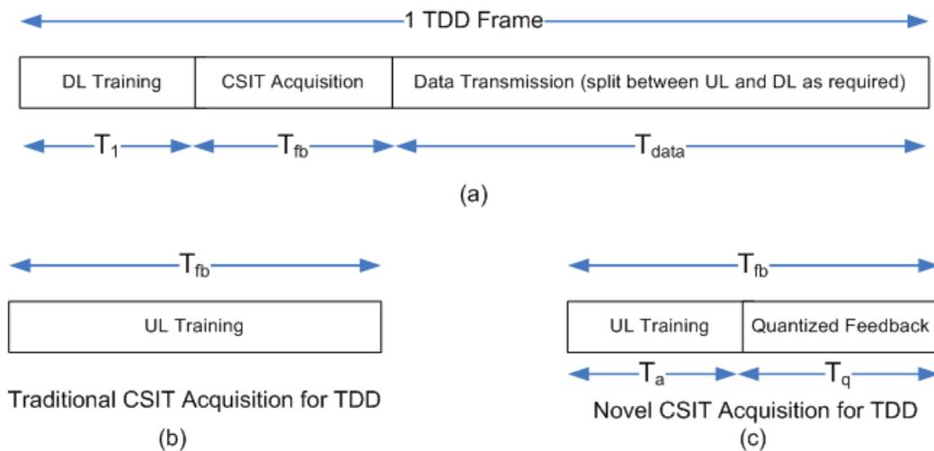
Fig. 1. (a) One TDD Frame; (b) Traditional CSIT Acquisition Setup for TDD systems; (c) Novel CSIT Acquisition Strategy for TDD systems: Total feedback length is divided between UL training and quantized feedback phases.
