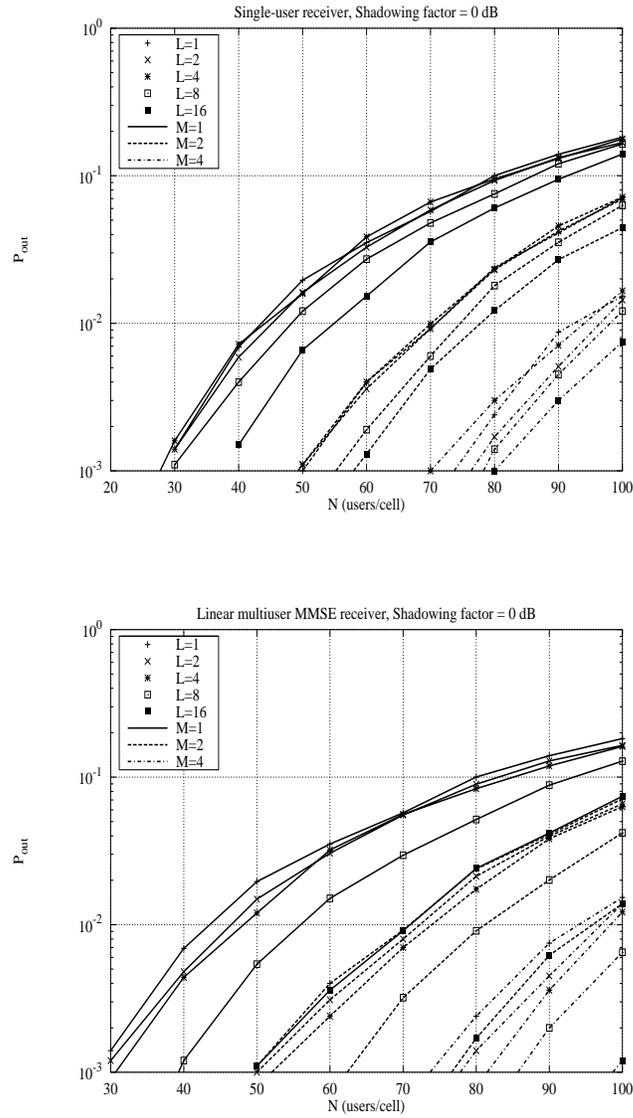
**Figure 1.5**  $P_{out}$  vs.  $N$  for fixed  $\rho/L = 7.7 \cdot 10^{-3}$ , for the single-user receiver (above) and for the linear MMSE multiuser receiver (below) with interleaving depths  $M = 1, 2, 4$ , spreading factors  $L = 1, 2, 4, 8, 16$  and ideal power control ( $\sigma_{sh} = 0$  dB).
