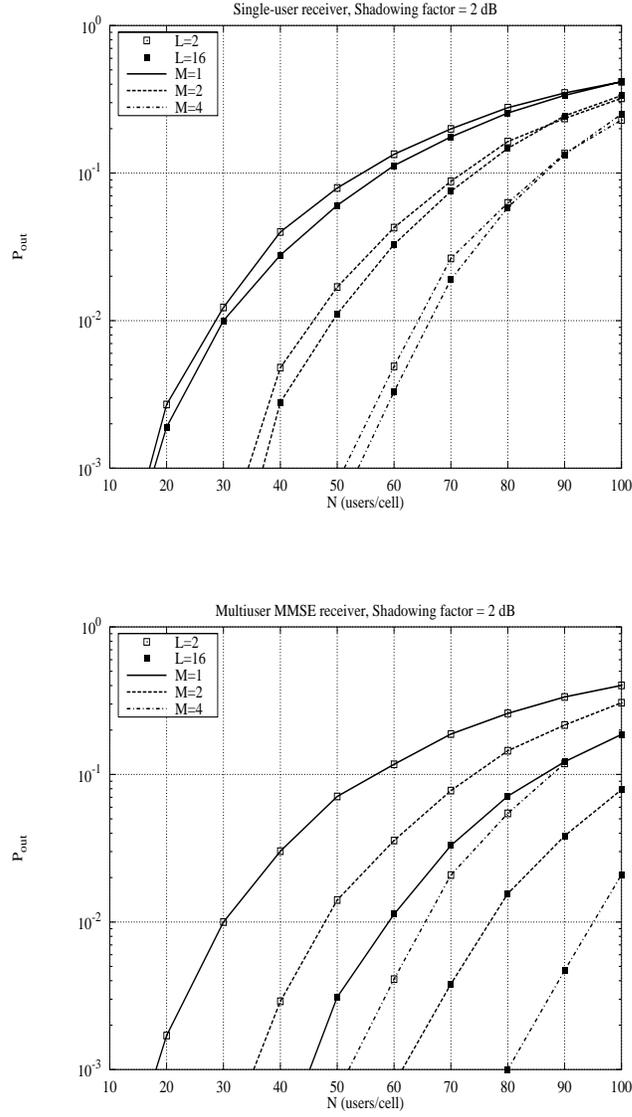
**Figure 1.6**  $P_{out}$  vs.  $N$  for fixed  $\rho/L = 7.7 \cdot 10^{-3}$ , for the single-user receiver (above) and for the linear MMSE multiuser receiver (below) with interleaving depths  $M = 1, 2, 4$ , spreading factors  $L = 2, 16$  and residual shadowing factor  $\sigma_{sh} = 2$  dB.
