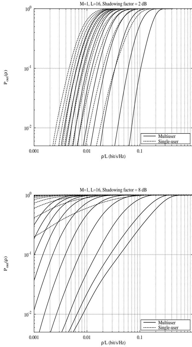
**Figure 1.3**  $P_{\text{out}}(\rho)$  vs.  $\rho/L$  for  $M = 1$ ,  $L = 16$ , with residual shadowing factor  $\sigma_{\text{sh}} = 2$  dB (above) and  $\sigma_{\text{sh}} = 8$  dB (below). Curves for  $N = 10, 20, \dots, 100$  users are shown. For each family of curves, the rightmost corresponds to  $N = 10$  and the leftmost to  $N = 100$ .
