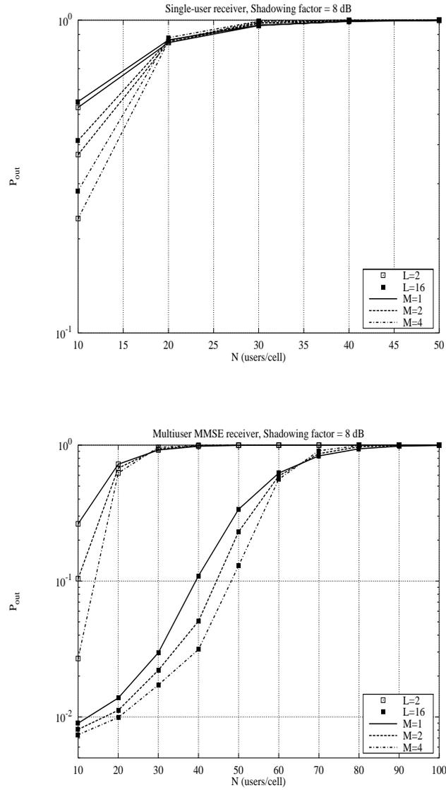
**Figure 1.7**  $P_{out}$  vs.  $N$  for fixed  $\rho/L = 7.7 \cdot 10^{-3}$ , for the single-user receiver (above) and for the linear MMSE multiuser receiver (below) with interleaving depths  $M = 1, 2, 4$ , spreading factors  $L = 2, 16$  and residual shadowing factor  $\sigma_{sh} = 8$  dB.
