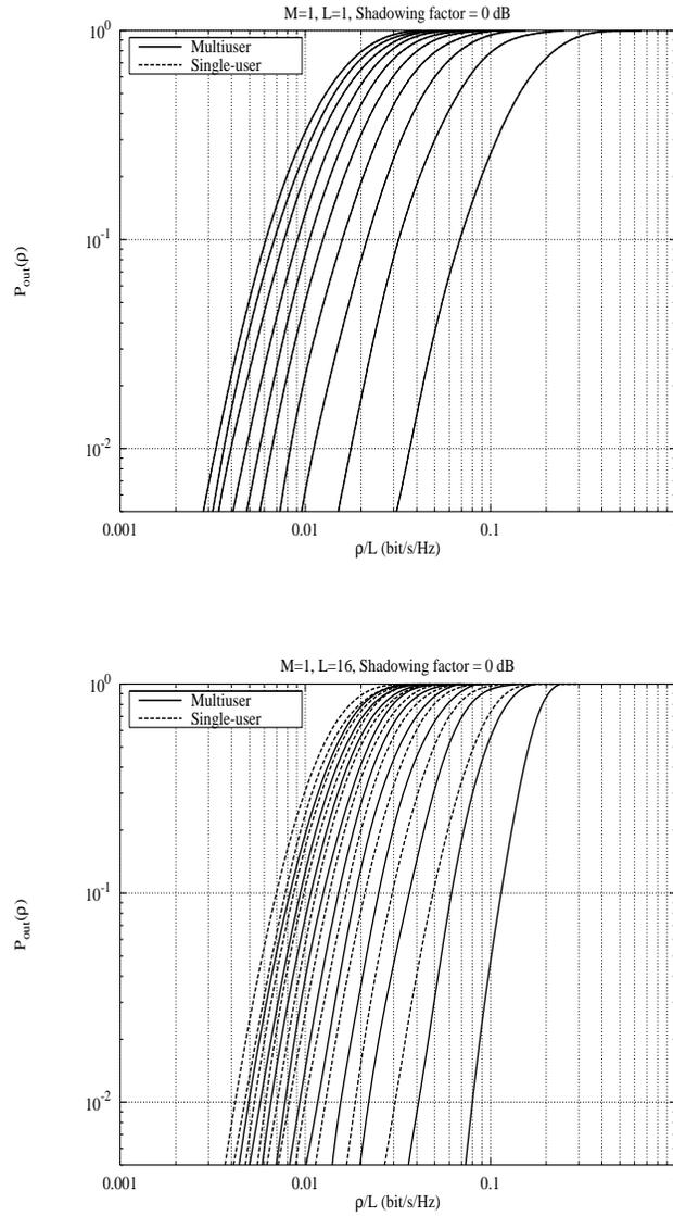
**Figure 1.2**  $P_{\text{out}}(\rho)$  vs.  $\rho/L$  for  $M = 1$ ,  $L = 1$  (above) and  $L = 16$  (below). Curves for  $N = 10, 20, \dots, 100$  users are shown. For each family of curves, the rightmost corresponds to  $N = 10$  and the leftmost to  $N = 100$ .
