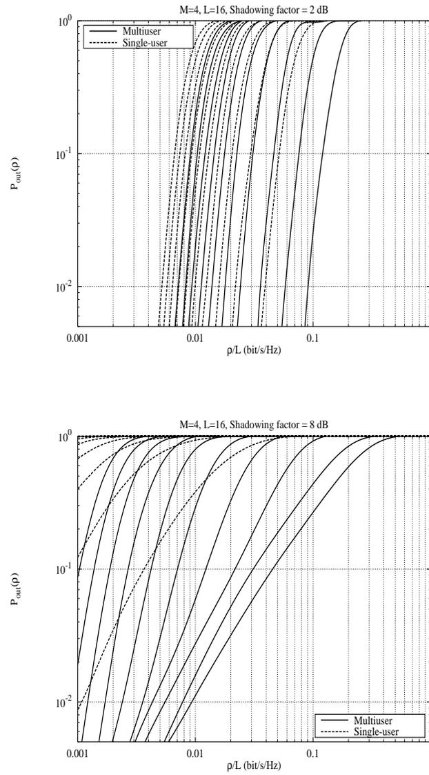
**Figure 1.4**  $P_{\text{out}}(\rho)$  vs.  $\rho/L$  for  $M = 4$ ,  $L = 16$ , with residual shadowing factor  $\sigma_{\text{sh}} = 2$  dB (above) and  $\sigma_{\text{sh}} = 8$  dB (below). Curves for  $N = 10, 20, \dots, 100$  users are shown. For each family of curves, the rightmost corresponds to  $N = 10$  and the leftmost to  $N = 100$ .
