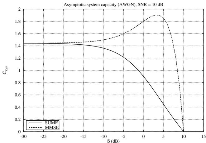
**Figure 1.1** System capacity vs.  $\beta$ , the signal-plus-interference to noise ratio at the receiver output for SNR= 10 dB, a single-user matched-filter receiver (continuous line) and a linear MMSE receiver (dotted line). The channel is ideal AWGN.
