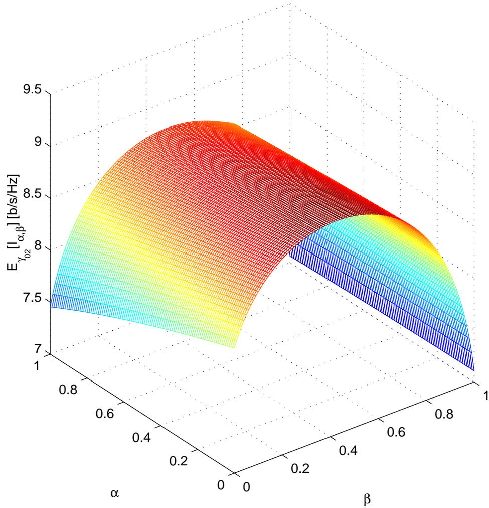
Figure 5: Expected sum-rate seen by mobile 1 (distributed processing) when the mobile 2 is located at (0.1,0) in linear network and SNR equal to 10 dB. The relations in (10) give (0,0.447) as optimal power allocation for mobile 1, therefore it doesn't cooperate.
