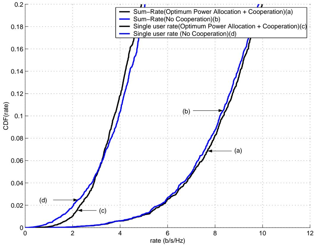
Figure 7: Outage capacity in centralized case and symmetric network in which we consider equal channel gains ( $\sigma^2 = 1$ ) : In this situation, individual users's worst-case rates are slightly improved, while the sum rate is almost unchanged.
