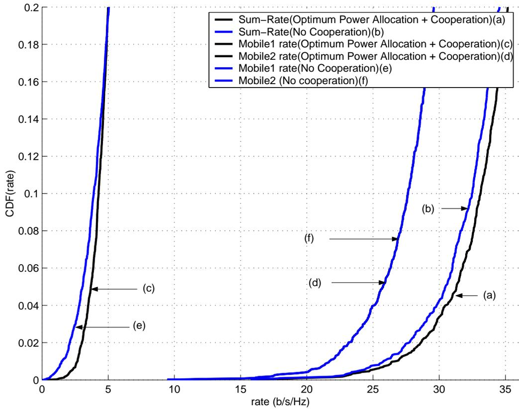
Figure 10: Outage capacity in centralized case and asymmetric network with user 2 located at  $(0.9,0)$ , i.e, close to the destination; both the sum-rate and user 1's rate benefit from the cooperation, while user 2 almost never uses user 1 as a relay.
