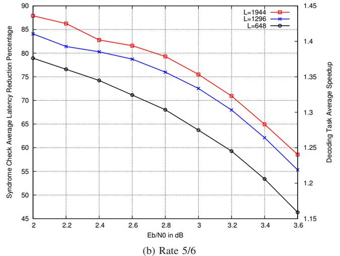
Fig. 9. Average latency reduction for the syndrome check process and overall decoding task speedup
