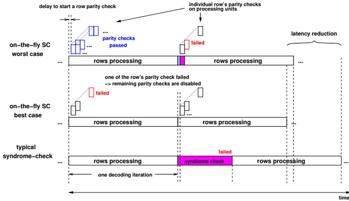
Fig. 3. Timing visualization for two consecutive decoding iterations
