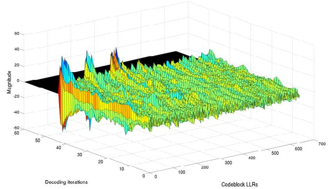
Fig. 2. LLRs magnitude evolution as a function of decoding iterations
