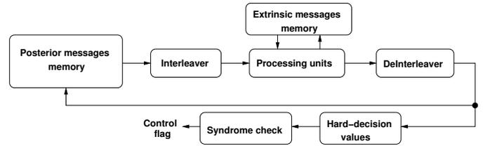
Fig. 7. Canonical decoder architecture
