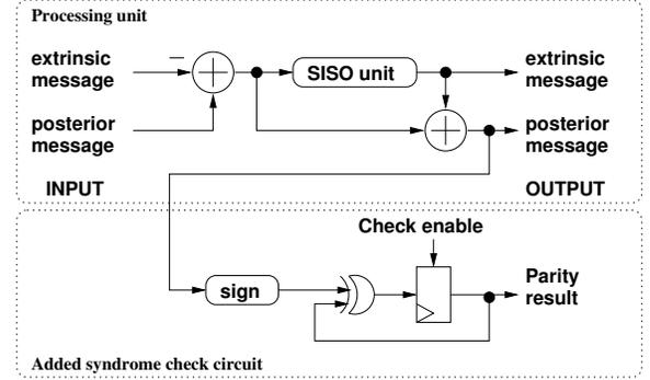
Fig. 8. Processing unit with syndrome check option
