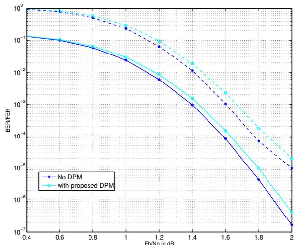
Fig. 11. Error-correcting performance: BER solid lines, FER dashed lines
