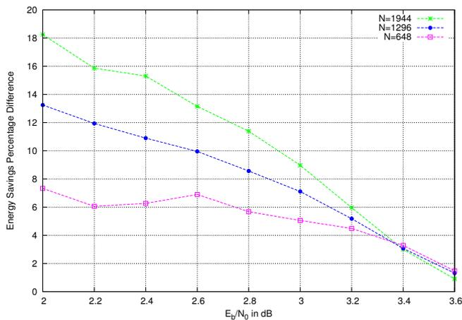
Fig. 13. Difference on savings between online and offline algorithms
