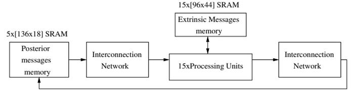
Fig. 7. LDPC decoder architecture
