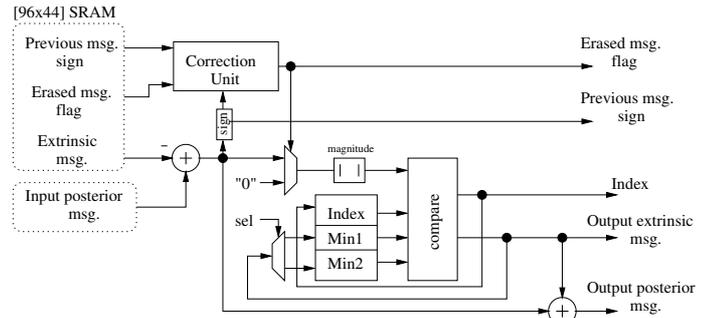
Fig. 8. Architecture of processing unit
