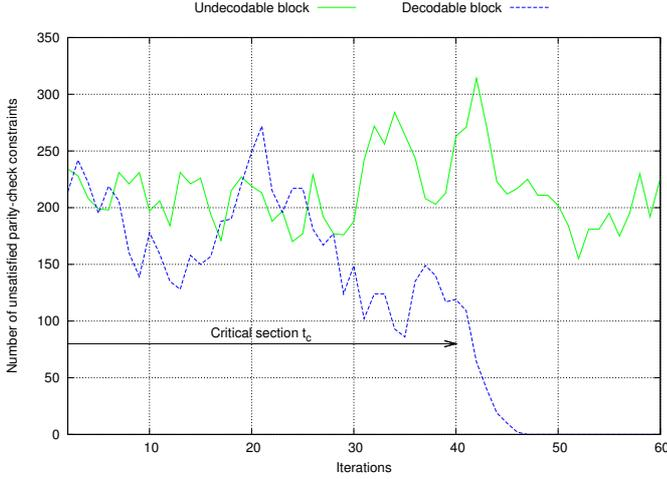
Fig. 3. Convergence metric for a decodable/undecodable block
