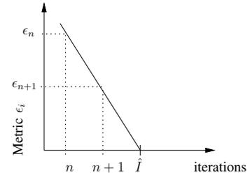
Fig. 4. Estimation of decoding effort by linear approximation
