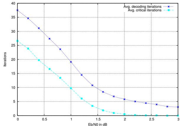
Fig. 10. Average decoding and critical iterations
