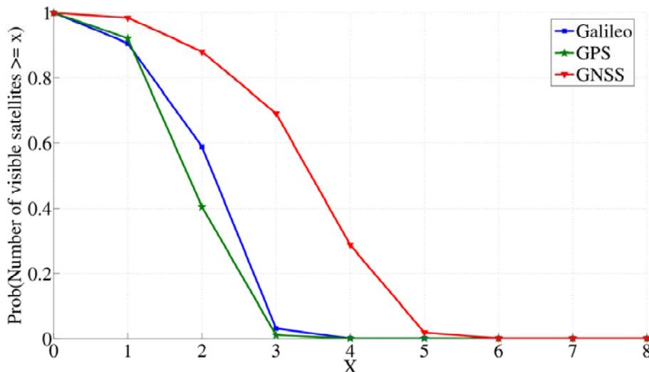
Figure 4 CDF of visible satellites in an urban canyon.
