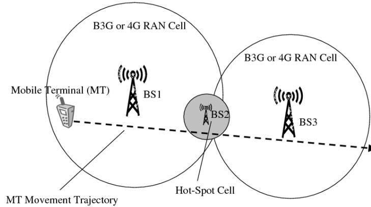
Figure 1 Location based horizontal (intra-system) or vertical (inter-system) handover.
