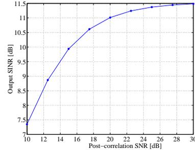
Figure 4: Optimum output SINR vs. input SNR
