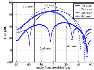
Figure 3: Radiation patterns after optimization
