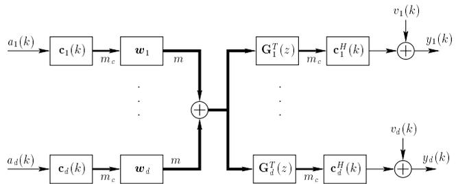
Figure 1: Transmission filters channels and RAKE receivers for  $d$  users
