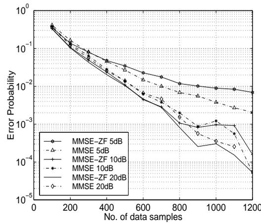
Figure 5: Error rate performance for spreading factor, P=16, and K=5 users.
