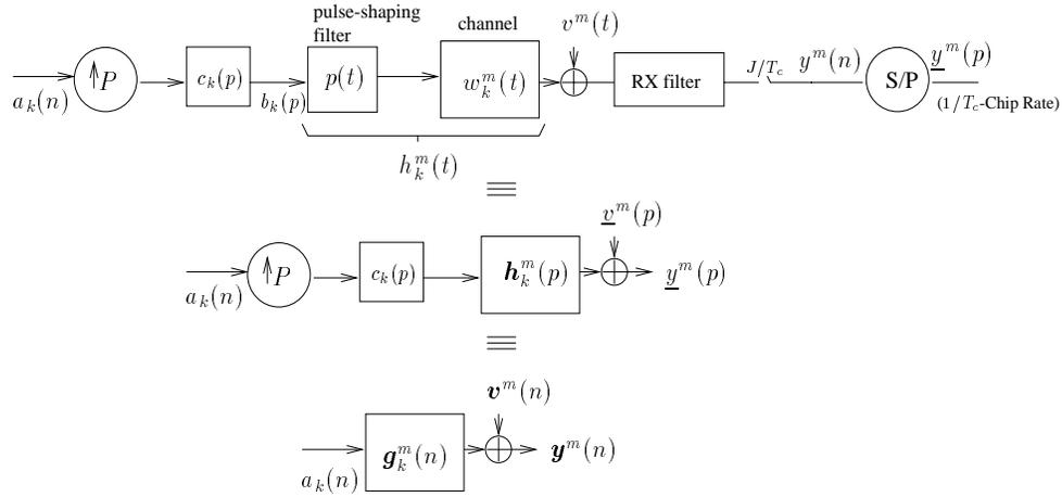
Figure 1: Signal model in continuous and discrete time, showing only the contribution from one user.
