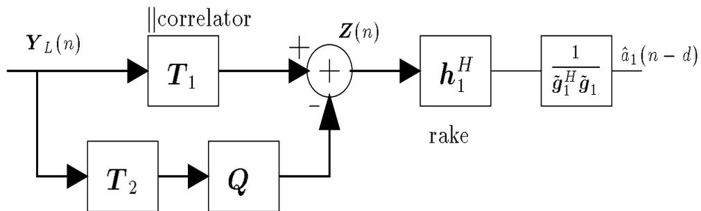
Figure 4: GSC implementation of the MMSE-ZF receiver.
