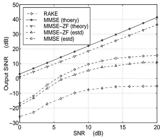
Figure 7: Output SINR performance of different receivers in near-far conditions for spreading factor, P=16, and K=5 users.
