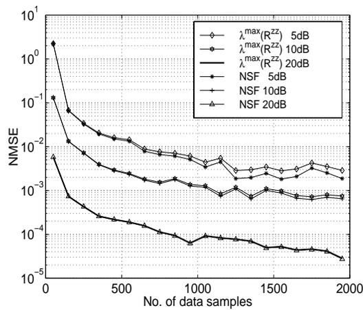
Figure 6: Channel estimation performance for spreading factor, P=16, and K=5 users.
