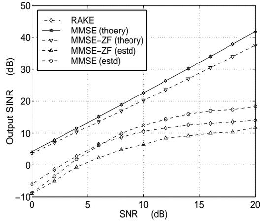
Figure 8: Output SINR performance of different receivers in power-controlled conditions for spreading factor,  $P=16$ , and  $K=5$  users.
