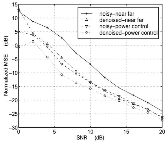
Figure 9: Normalized channel estimation MSE for the denoised and non-denoised  $R_{YY}$ , for spreading factor,  $P=16$ , and  $K=5$  users
