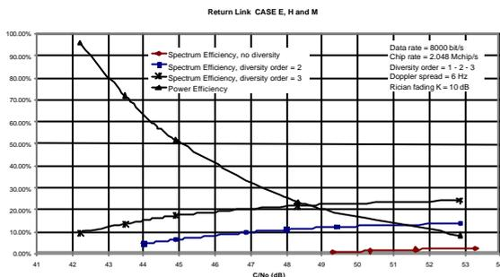
Figure 6: Reverse link power and spectral efficiency for single and dual path diversity.
