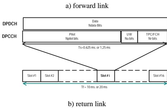
Figure 1: *Frame Structure of the Forward and Return Link Dedicated Physical Channels (DDPCH/DCPCH).*
