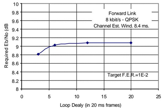
Figure 7: Required Eb/No for F.E.R.= $10^{-2}$  as a function of the loop delay (power control gain step=0.5 dB) for a slow fading case (Doppler spread= 6 Hz).
