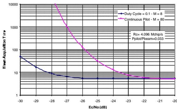
Figure 2: Forward link mean acquisition time (ms.) versus pilot thermal  $E_c/N_0$  for a continuous and bursty pilot.
