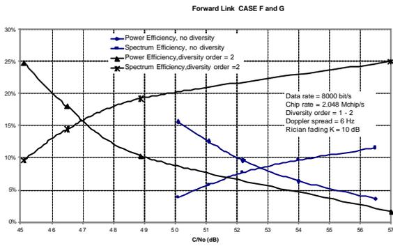
Figure 5: Forward link power and spectral efficiency for single and dual path diversity.
