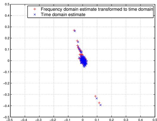
Fig. 4. IQ plot of the estimated impulse response of the reciprocity filter
