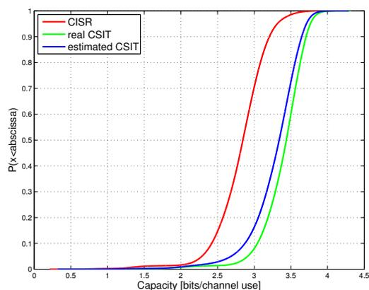
Fig. 5. CDF of the capacity of the MIMO channel at 10 dB SNR
