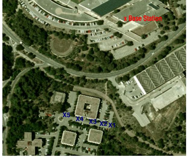
**Fig. 3.** Map of the measurement scenario. The position of the BS antenna as well as the five measurement points are indicated.
