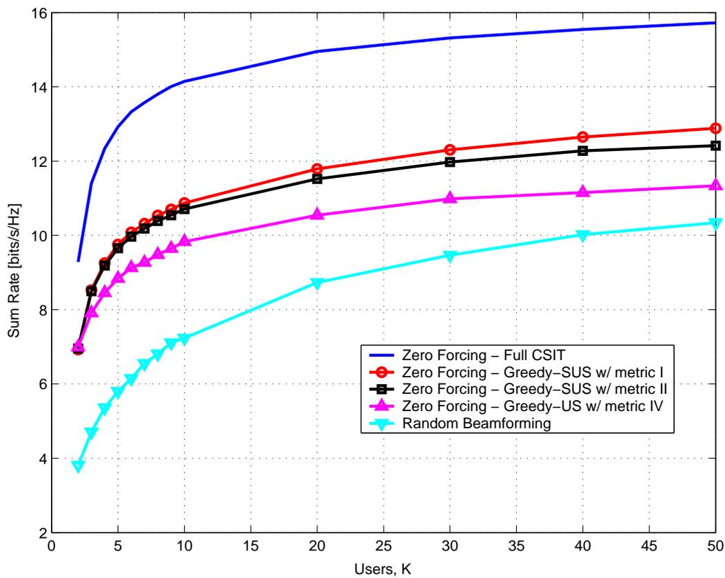
Fig. 3. Sum rate versus the number of users for different approaches with  $SNR = 20$  dB,  $M = 2$  transmit antennas and limited 10-bit total feedback bits where  $B = 5$  bits are used for codebook indexing and  $(10 - B)$  bits for CQI quantization. For metric IV, 2 bits are used for quantization of the channel norm and 3 bits for the alignment.
