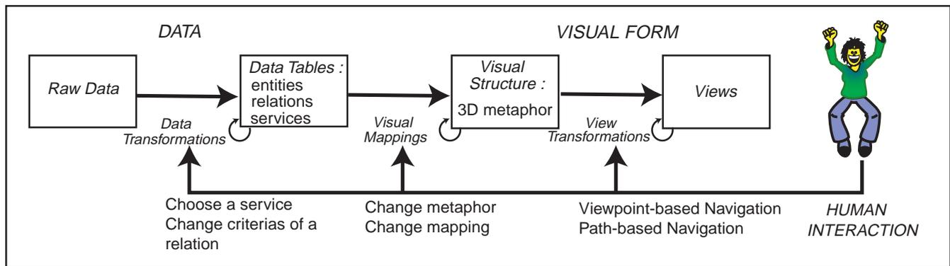
Figure 6: Reference model from Card et al <sup>6</sup> applied to our system
