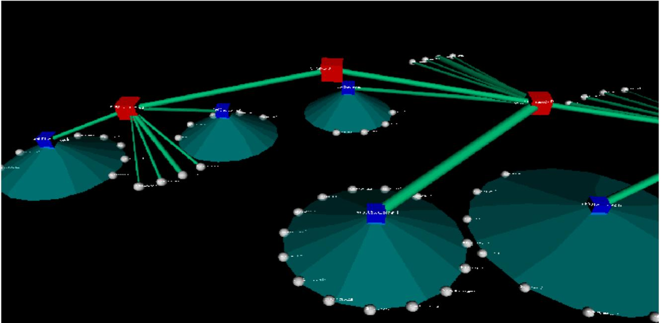
Figure 8 : Topological view of a subpart of the Eurecom Institute network using a cone tree visualization model. The width of the links is dependent on network traffic and the shading is related to the packet loss for that link. The transparency of a cone is dependent on the collision rate of the hub it is associated with.
