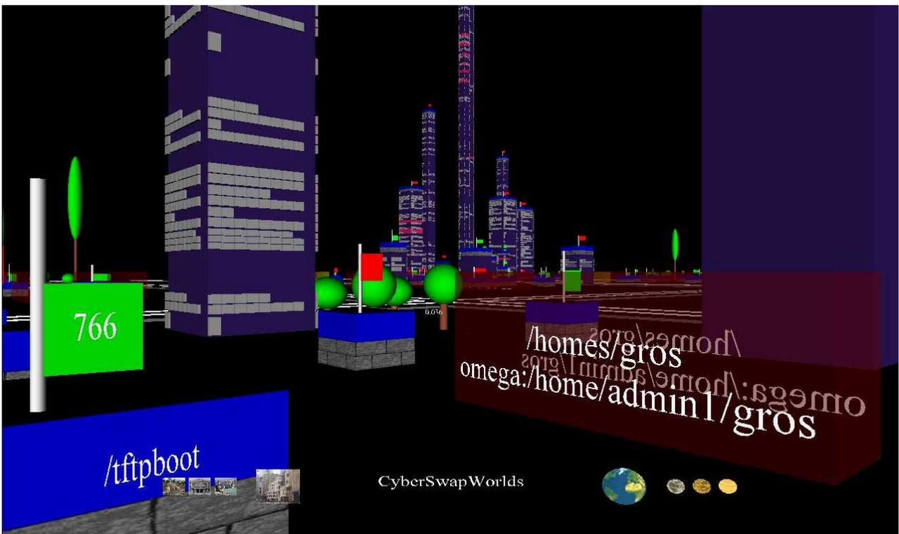
Figures 4 and 5 : NFS related information of the Eurecom network mapped on a city metaphor. Each district is a workstation where buildings represent disks. Each storey of a building represents a NFS client which is mounting this disk. The number of windows of a floor represents the number of file handles of the client. More details about mapping can be found on our Web site ([www.eurecom.fr/~abel/cybernet/](http://www.eurecom.fr/~abel/cybernet/))
