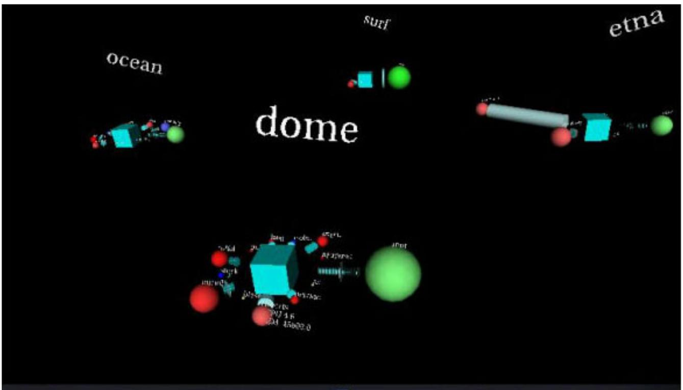
Figure 9 : This picture shows several workstations with its users around it using a solar system metaphor. Each user is a sphere. The sphere's color corresponds to the unix group of the user, the size to the memory the user is using and the color's intensity to the CPU time. Between the users (sphere) and the workstation (cube), user's processes are displayed as cylinders. The cylinder's visual parameters follow the same guideline as sphere in order to keep coherency (size → memory, color → cpu)
