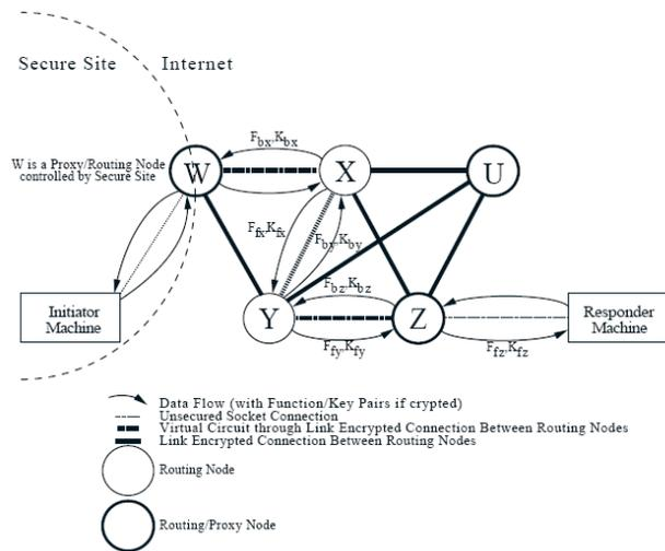
Fig. 5. Onion routing virtual circuit [16]
