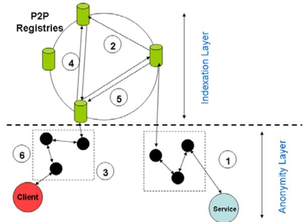
Fig. 9. Architecture for a secure distributed registry-based service discovery
