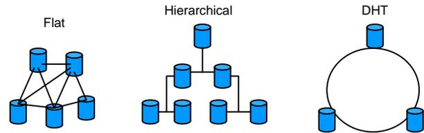
Fig. 1. Alternative architectures for distributed registries
