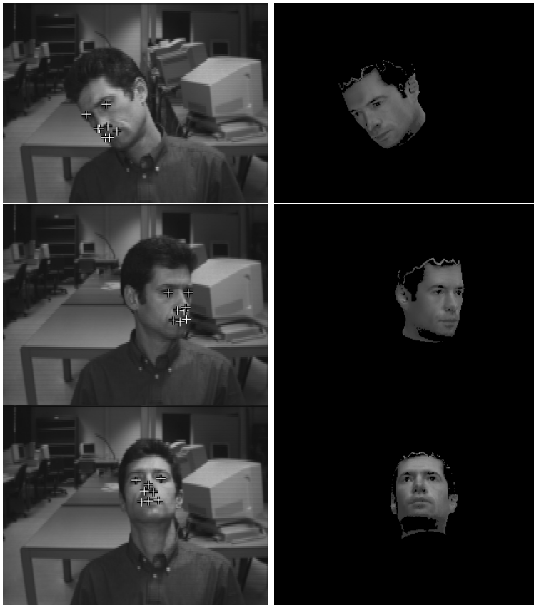
Figure 11: Head rotations supported by our face tracking system, without markers and uniform lighting.
