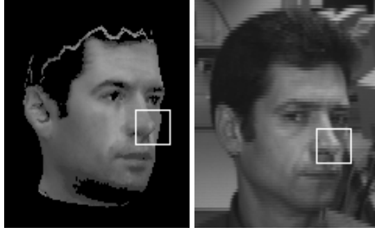
Figure 6: For this typical rotation, the synthetic background used by the encoder appears in the tracked nose area. As its pixels would lead to a wrong match in the real image, they are discarded by the tracker for the computation of the temporal gradient \mathbf{I}_t . As a result, the tracker restricts itself only to the potential face pixels in the video frame, and is able to find the right match despite the unknown background in the real world.
