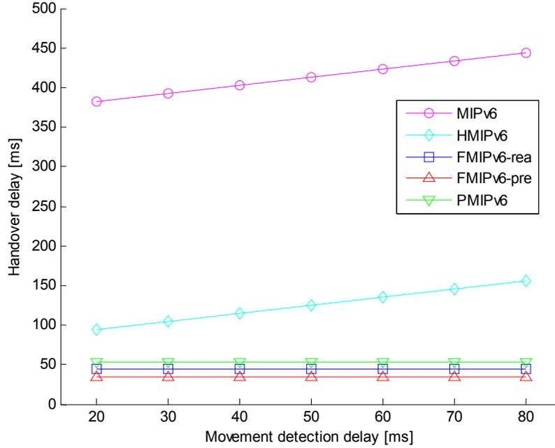
**Figure 7. Handover delay vs. movement detection delay**
