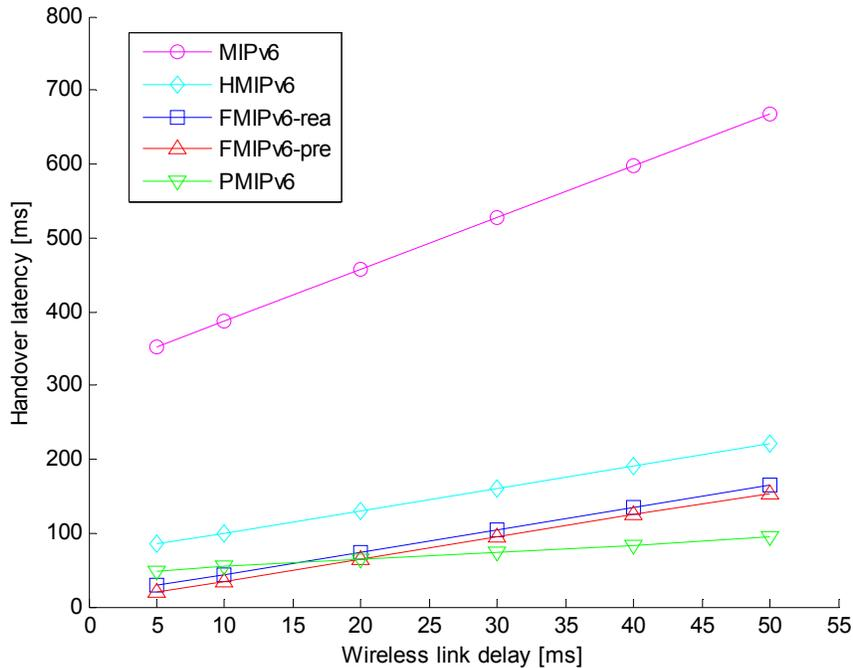
**Figure 6. Handover latency vs. wireless link delay**
