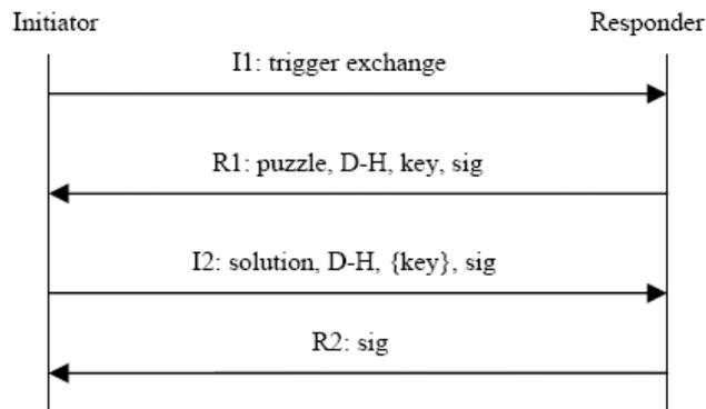
Figure 13. HIP Base Exchange
