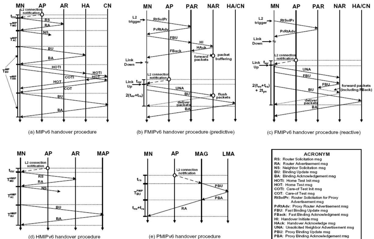
Figure 4. Handover procedure for each protocol.
