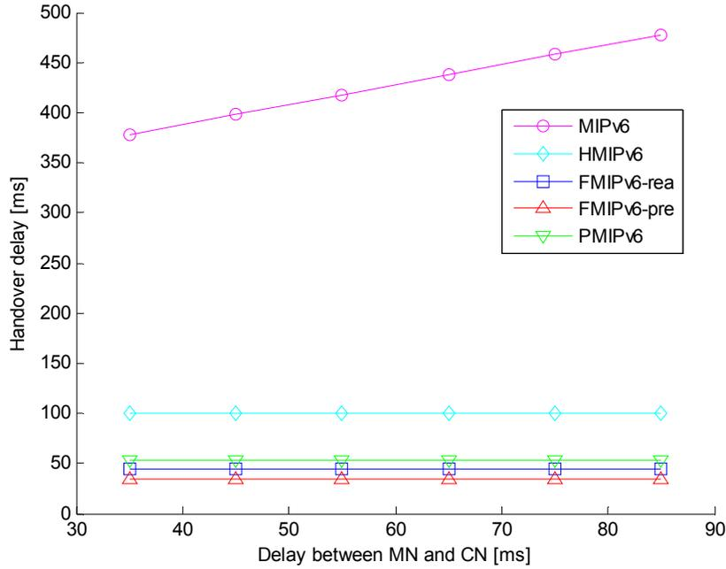
**Figure 8. Handover latency vs. delay between MN and CN**
