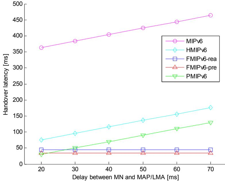
**Figure 9. Handover latency vs. delay between MN and MAP/LMA**
