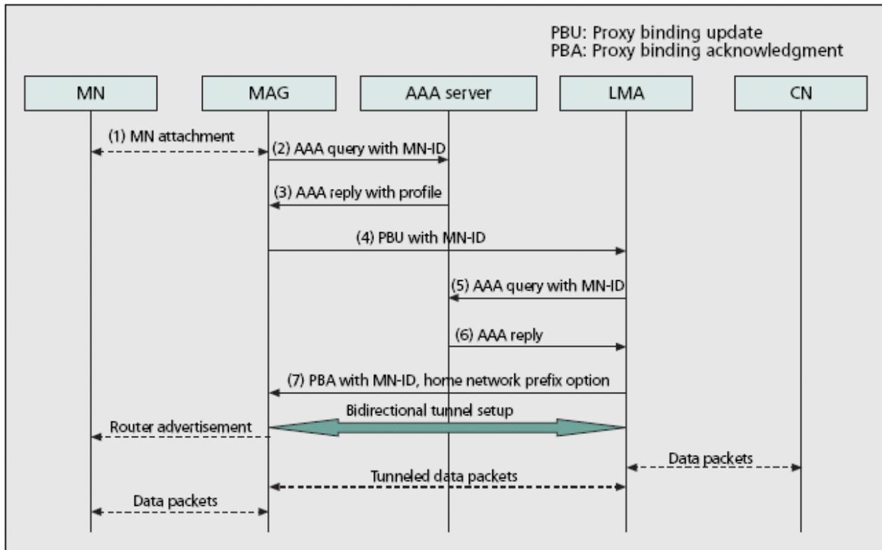
Figure 3. Message flow in PMIPv6
