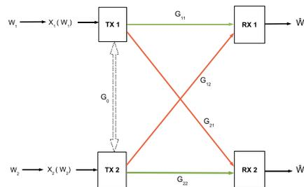
Figure 1. Interference channel with possible transmitter cooperation.
