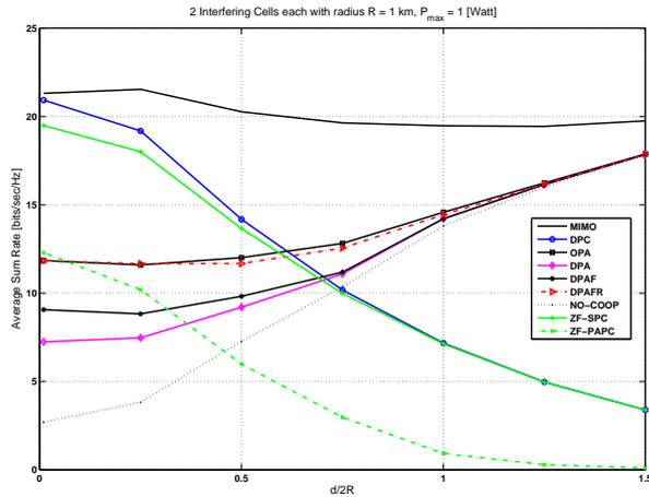
Figure 4. Average sum of rates versus  $d/2R$  for circular cell layout.
