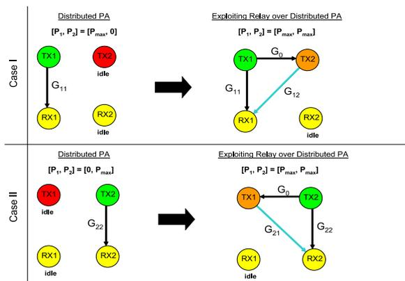
Figure 2. Two cases for which relaying mechanism is used after DPA.
