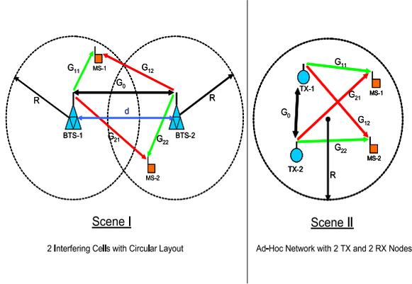
Figure 3. Two Simulation Scenes considered: Scene I is 2 interfering cell with circular layout and Scene II is Ad-Hoc network.
