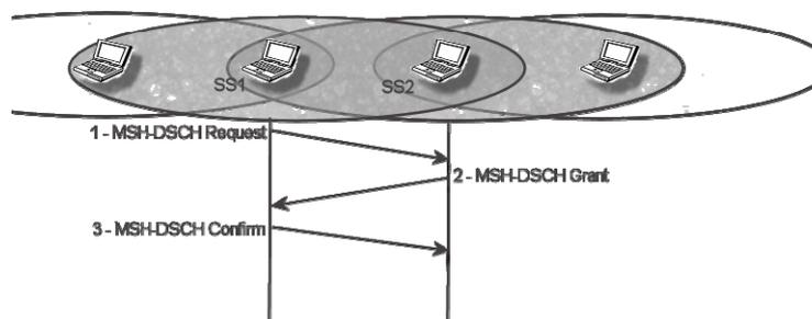
Fig. 4 - Distributed Scheduling Three Way Hand Shake.
