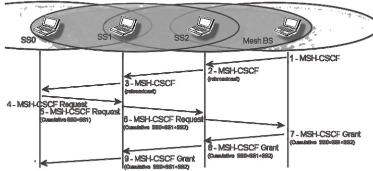
Fig. 3 - A message flow example for the centralized scheme.
