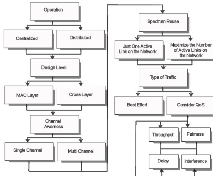
Fig. 5 - Proposed classification for WiMax mesh mode CAC algorithms.
