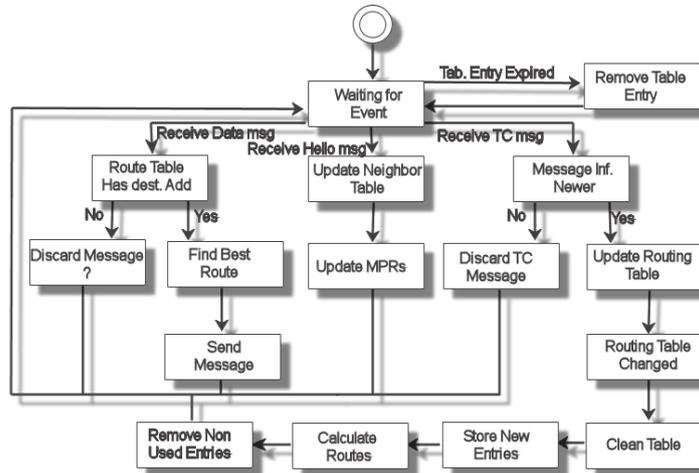
Fig. 2 - Simplified OLSR intermediate node diagram.
