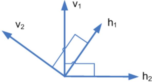
Fig. 2. Channel Projections and corresponding ZF vectors for users 1 and 2 in 2-D null space of all other users' channel vectors
