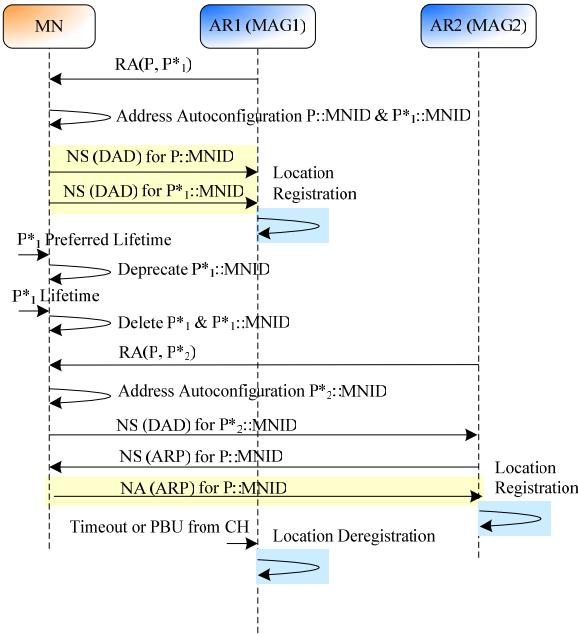
**Figure 6. Example of Enhanced Network-based IP-Layer Movement Detection**
