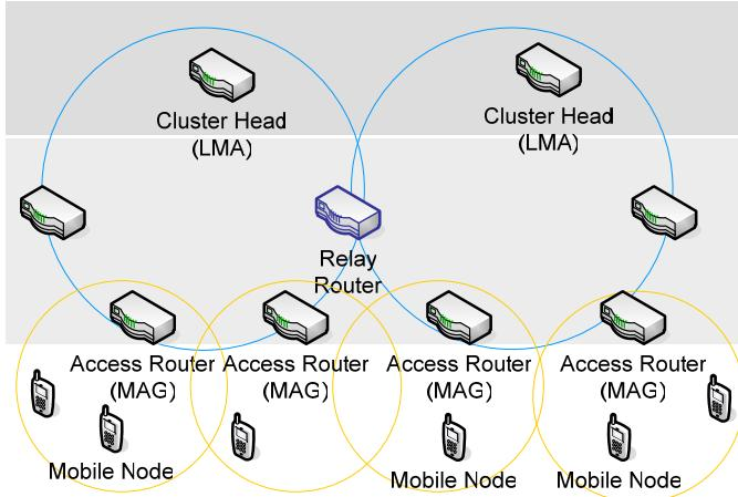
**Figure 3. Scalability with Cluster-based Architecture**
