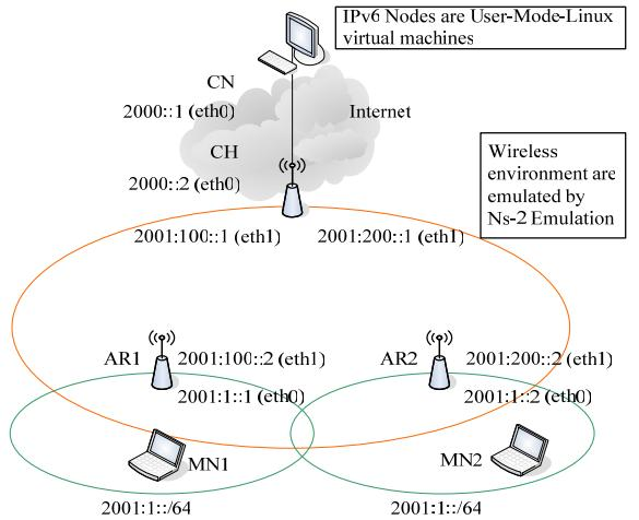
Figure 11. Virtual Wireless Mesh Testbed
