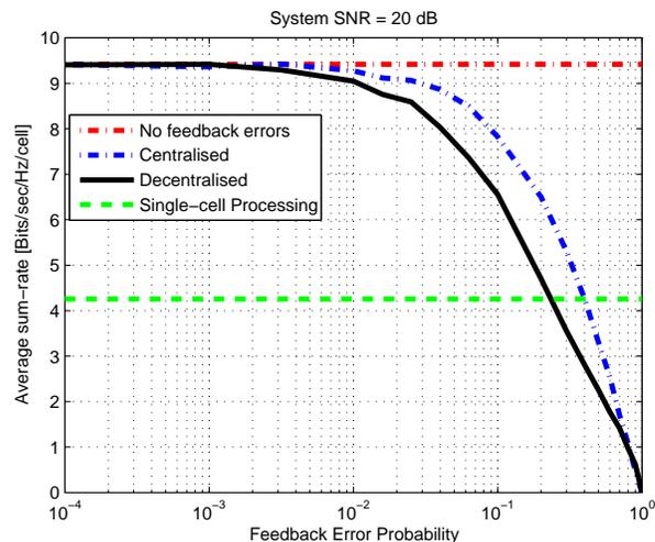
Fig. 4. Digital feedback: a plot of the average sum-rate as a function of the feedback error probability for the decentralised and the centralised framework respectively.
