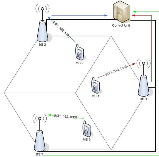
Fig. 1. Phase 2 of the existing centralised framework: MSs feedback their CSI to their Master BS and local CSI is exchanged with a Control Unit.
