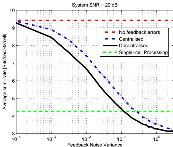
Fig. 3. Analogue feedback: a plot of the average sum-rate as a function of the feedback error noise variance for the decentralised and the centralised framework respectively.
