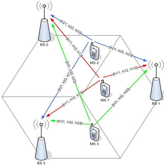
Fig. 2. Phase 2 of the proposed decentralised framework: MSs feed back their CSI to all cooperating BSs.
