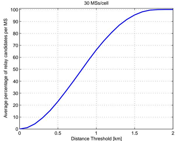
Fig. 1. A plot of the average percentage of considered relay candidates per MS as a function of the distance threshold.
