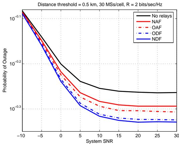
Fig. 3. A plot of the probability of outage versus the System SNR under the presence of ICI.
