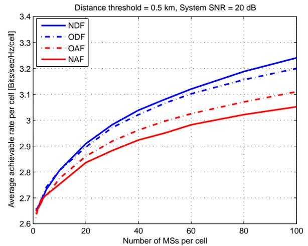
Fig. 5. A plot of the average sum-rate per cell versus the number of cell users.
