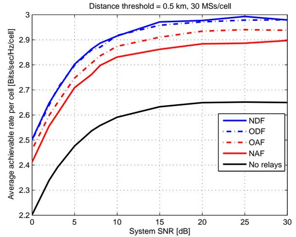
Fig. 4. A plot of the average sum-rate per cell versus system SNR.
