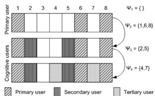
Figure 2 One primary user and two cognitive users in a spectrum-pooling system with eight sub-bands
