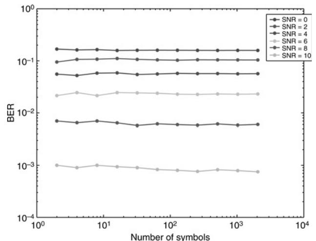
Figure 3 BER against number of symbols ( $M$ ) in decibel for BPSK in AWGN using power detection where SNRs are in decibel
