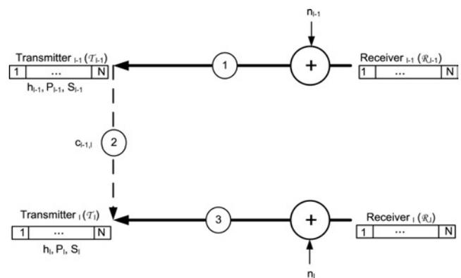
Figure 1 Cognitive radio channel in a wideband/multiband context with  $N$  sub-bands
