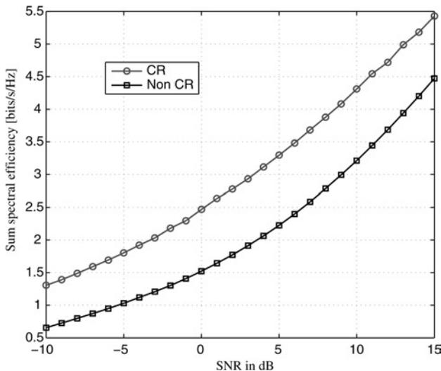
Figure 7 Sum spectral efficiency of a system using CR and a traditional system (non-CR) for  $N = 512$
