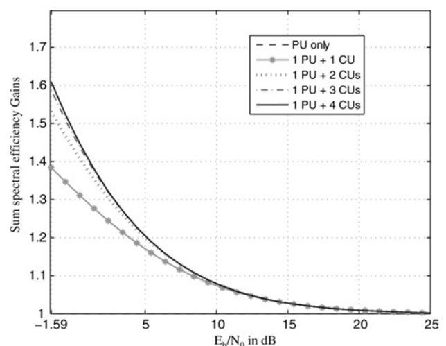
**Figure 6** Sum spectral efficiency gains of the system with one primary user and four CUs
