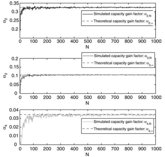
Figure 8 Convergence of band factor gains at SNR = 0 dB
