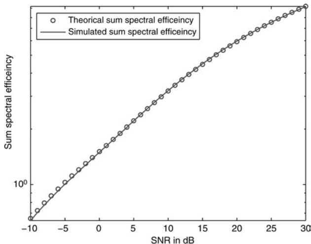
**Figure 4** Comparison between theoretical expression of the sum spectral efficiency in (31) and simulated one in (17) for  $L = 5$  and  $N = 16$
