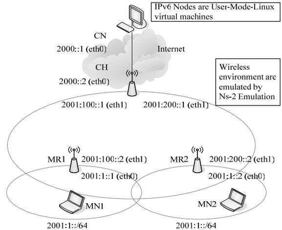
Figure 6. Virtual Wireless Mesh Testbed
