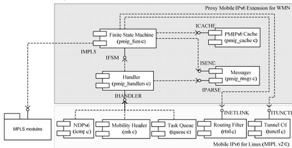
Figure 5. PMIPv6 Software Architecture
