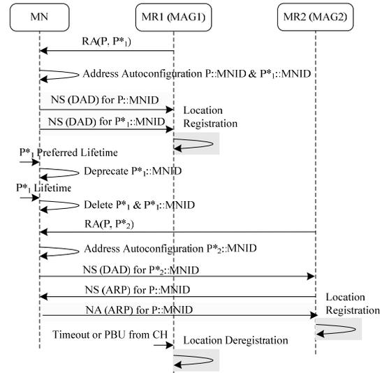
**Figure 4. Example of Enhanced Network-based IP-Layer Movement Detection**
