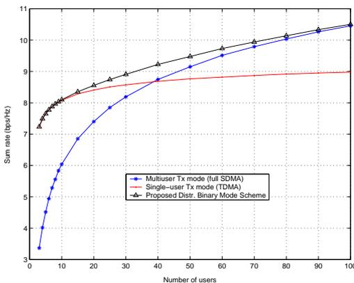
**Fig. 2.** Sum rate versus the number of users for binary mode selection with  $M = 3$  and average SNR = 20dB.
