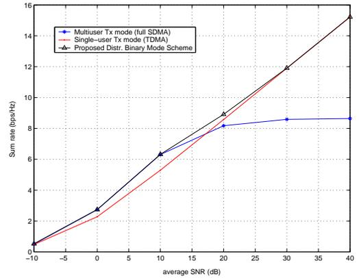
**Fig. 3.** Sum rate versus average SNR for binary mode selection with  $M = 3$  and  $K = 30$  users.
