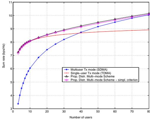
**Fig. 1.** Sum rate versus the number of users for distributed multi-mode scheme with  $M = 3$  and average SNR = 20dB.
