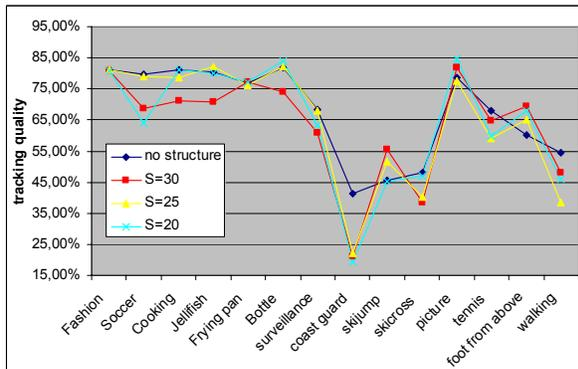
**Figure 6: tracking quality with and without the use of the structure for 14 videos sequences. Various threshold  $S$  settings are shown.**
