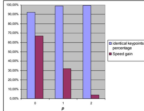
**Figure 4: Influence of the  $p$  parameter on the algorithm. The measures are the speed gain and the percentage of identical keypoints compared to the Harris extractor only. Each test is the mean of three executions for a structure of 1, 3, or 6 levels and  $S=20$ .**
