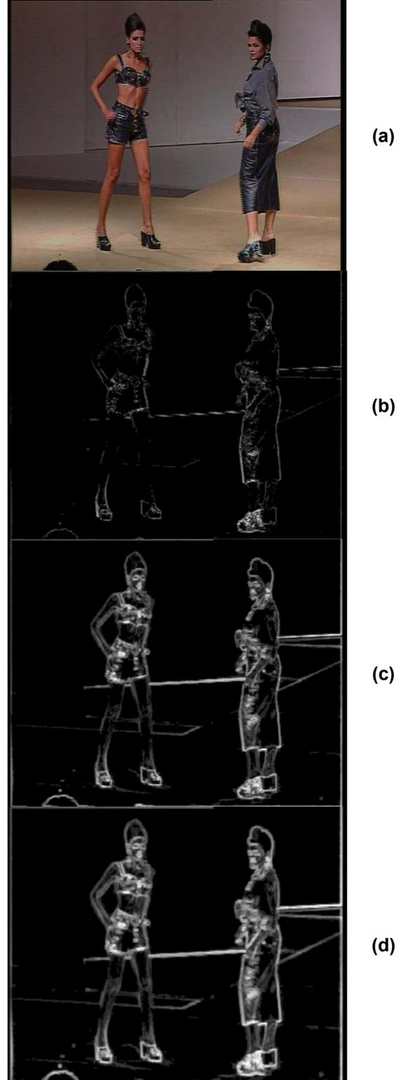
Figure 2: illustration of the Neighborhood parameter  $p$  influence. White pixels are pixels retained for keypoint extraction. (a) Analyzed image. Results for (b)  $p=0$  (c)  $p=1$  (d)  $p=2$ .
