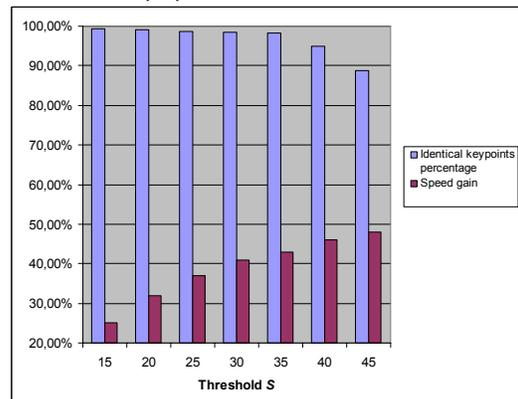
**Figure 5: Influence of the threshold  $S$  on the algorithm. The measures are the speed gain and the percentage of identical keypoints compared to the Harris extractor only. Each test is done with a 3 levels structure and  $p=1$ .**
