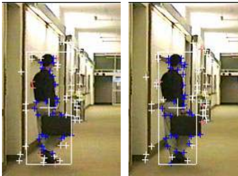
Figure 6: bounding box rescaling. Frames 7 and 8 of the “surveillance” sequence. The “object” keypoints are in blue, those of the “background” in white, undetermined keypoints are in red.
