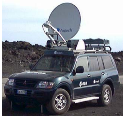
Figure 8: ESA Pajero and Temix EasyFlySat terminal
