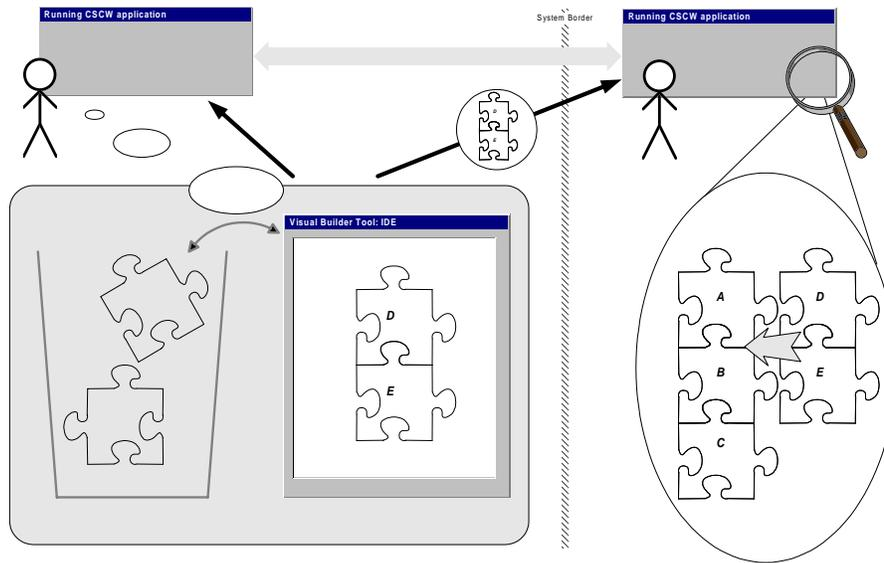
Figure 1. The two-step approach to tailor a CSCW application.
