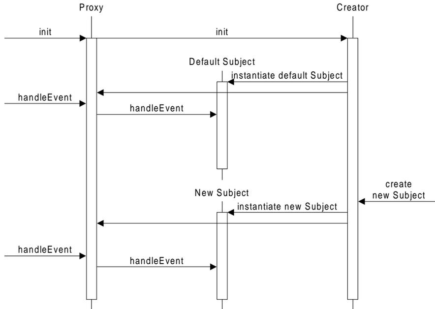
Figure 3. Interaction diagram for the Extensibility pattern.
