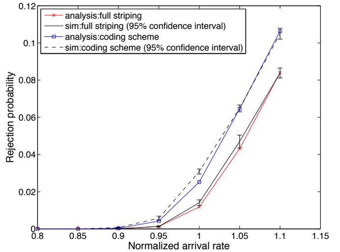
Fig. 1. Rejection probability with  $M = 128$ , Video encoding rate  $R_{enc} = 2Mbps$ , Upstream bandwidth  $B_{up} = 1Mbps$ , Size of Video  $L = 2Gbytes$ , Coding overhead  $\epsilon = 0.05$ , and Maximum number of simultaneous incoming connection  $y = 31$ .
