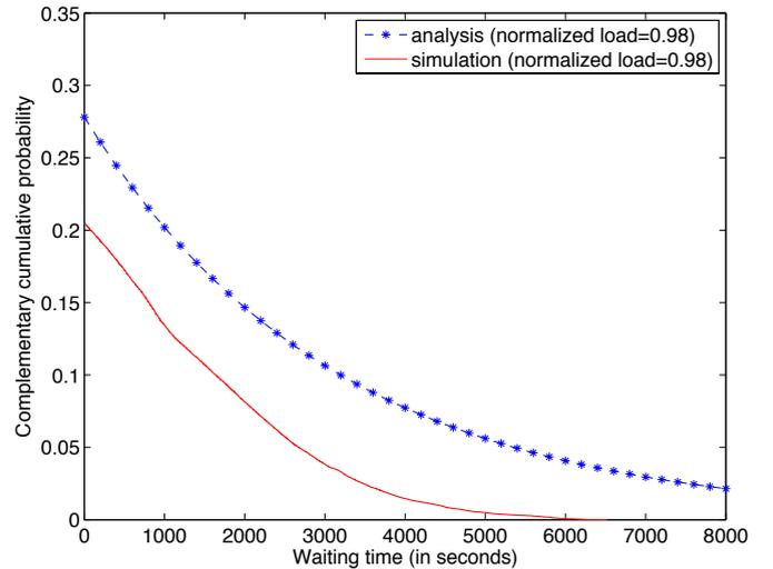
Fig. 2. Waiting time distribution for full striping with  $M = 128$ , Video encoding rate  $R_{enc} = 2Mbps$ , Upstream bandwidth  $B_{up} = 1Mbps$ , Size of Video  $L = 2Gbytes$  and a normalized load of  $\rho = 0.98$
