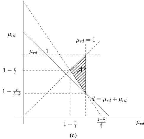
Fig. 5. The region  $\mathcal{A}^+$  for the long-term static channel for various cases. (a)  $\min(\mu_{sd}, \mu_{rd}) = \mu_{sd}$ . (b)  $\min(\mu_{sd}, \mu_{rd}) = \mu_{rd}$  and  $k \leq \lfloor l/2 \rfloor$ . (c)  $\min(\mu_{sd}, \mu_{rd}) = \mu_{rd}$  and  $\lfloor l/2 \rfloor < k \leq l-1$ .
