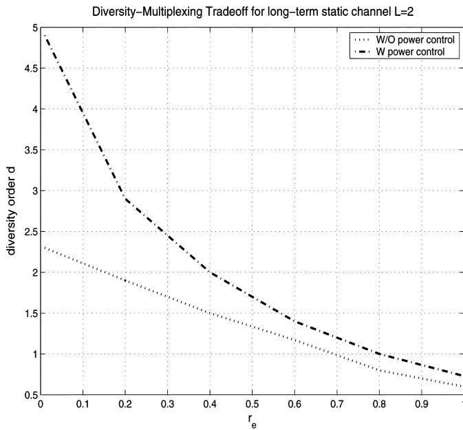
Fig. 4. The diversity-multiplexing tradeoff for  $L = 2$  for the long-term static channel with and without power control.
