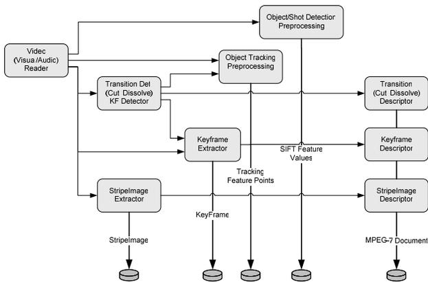
**Figure 2: Analyses module graph of the MediaAnalyze Tool**
