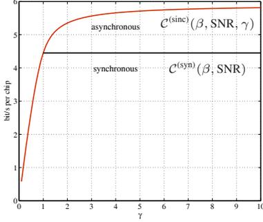
Fig. 1. Large system capacity per chip versus  $\gamma$  for  $\beta = 1$  and  $\frac{E_b}{N_0} = 10$  dB.
