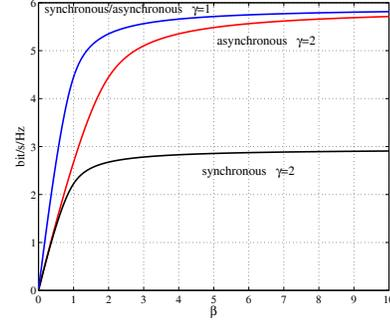
Fig. 2. Spectral efficiency versus  $\beta$  for  $\frac{E_b}{N_0} = 10$  dB.
