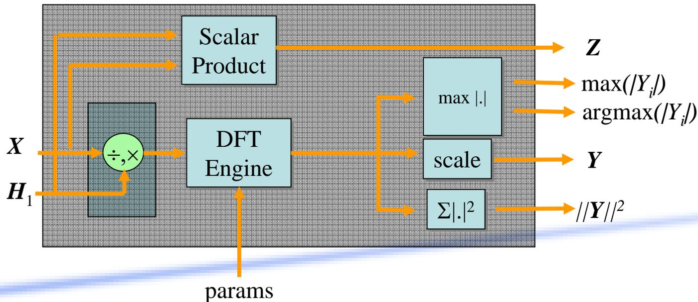
**Uses:** OFDMA : TX,RX,Ch Est,Frame Sync, Carrier phase offset compensation
