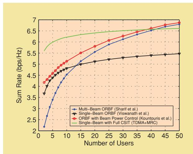
**[FIG3]** The sum rate is compared for random beamforming schemes with SINR feedback. Multibeam (SDMA) random beamforming outperforms the single-beam (TDMA) when the number of active users is sufficient. Power control over the random beams allows for a smooth transition between TDMA and SDMA. TDMA with full CSIT outperforms partial feedback schemes for a small number of users but fails to provide multiplexing gain when this number increases.
