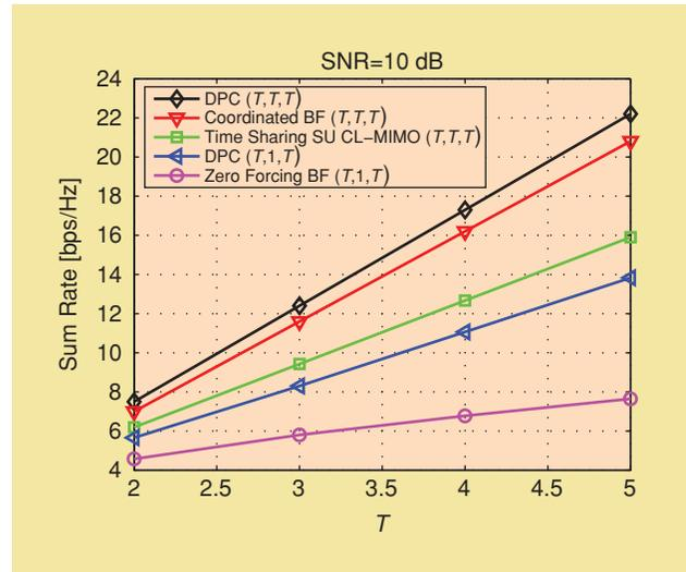
[FIG2] Ergodic sum capacity and achievable sum rate as a function of the number of users, the number of transmit/receive antennas.  $(T_1, T_2, T_3)$  denotes the number of transmit antennas at the BS, the number of receive antennas at the user, and the number of active users in the network, respectively. Coordinated BF refers to the method presented in [19].
